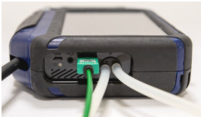
Fig. 38: Analyzer with pressure hoses and temperature plug
