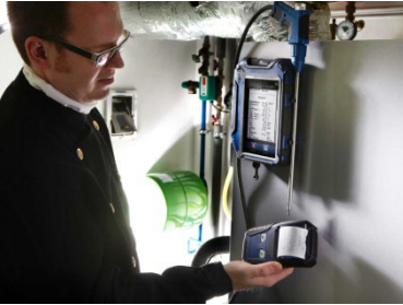
Fig. 35: Printing the readings of the Wohler A 550 INDUSTRIAL on the Thermalprinter Wohler TD 100.
